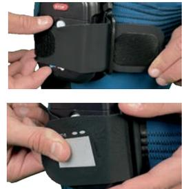
*Note: If the latch does not close into the loop of the Control Box, ensure that the Control Box is pushed in all the way. Do not force!*
