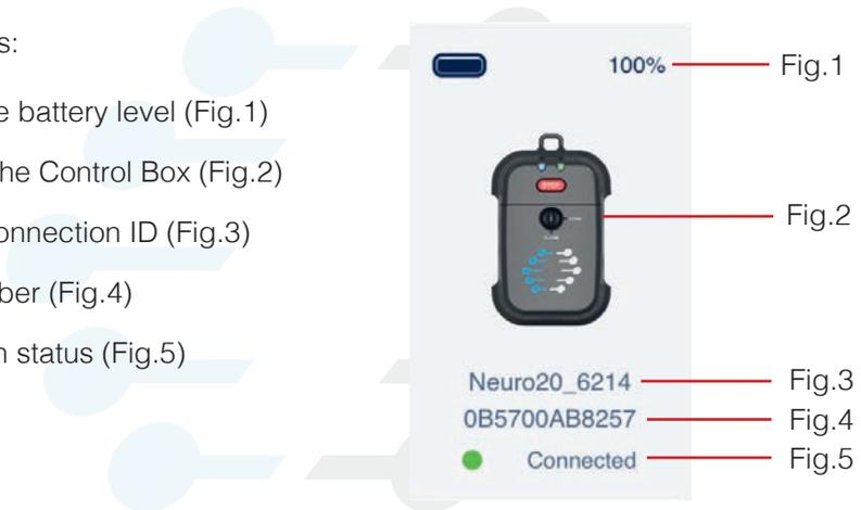
Battery Charge displays 100%, 50%, 25% and 10% levels.
